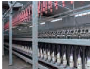
Bobbin rail with full bobbins is driven forward out of the FL
